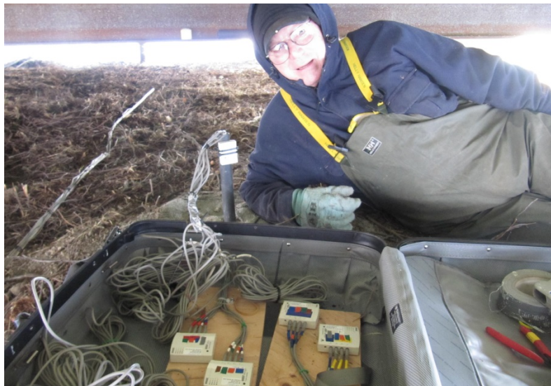
Figure 52. Willow House: HOBO thermistors installed, ready to place seasonal insulation.
