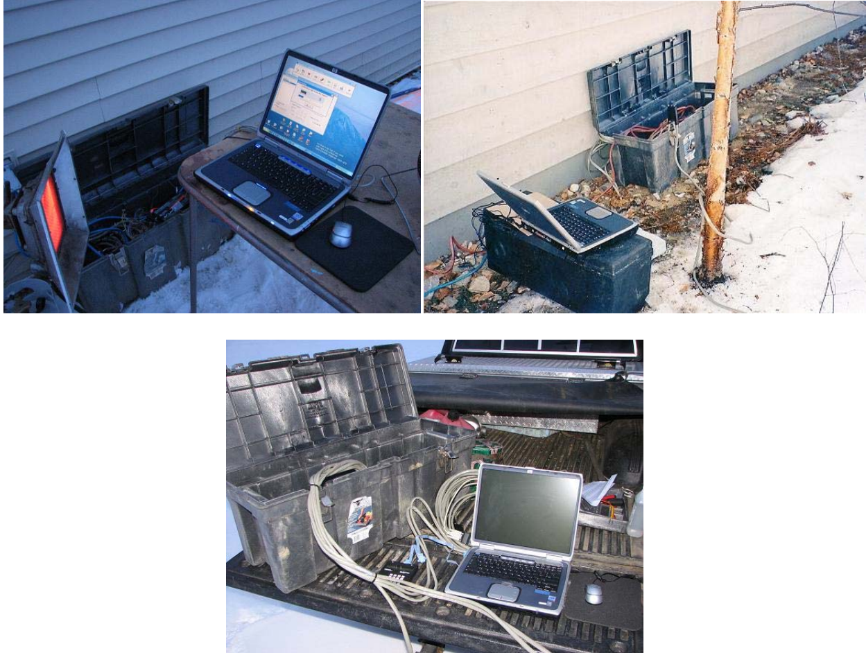
Figure 17. Fixed and mobile platforms for downloading data. (Top Left and Right) Hardwired dataloggers at two sites. (Bottom) A mobile station for Timberland, Bonita, Army and Violin sites.
